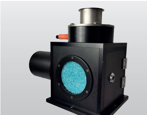
After completion of the measurement, which takes only fractions of a second, the sample material is discharged via a pneumatically controlled valve and added back to the process. Another special feature of the system is the laterally arranged measuring head. Long-term stable and durable light-emitting diodes are used as the light source. These last virtually the life of the device and do not need to be replaced.
