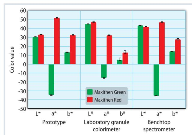
**Fig. 5.** Comparison of the L\*, a\*, b\* values of the developed prototype with different measuring devices on the two materials Maxithen Green and Maxithen Red: the prototype measures similar values as the benchtop spectrometer.
