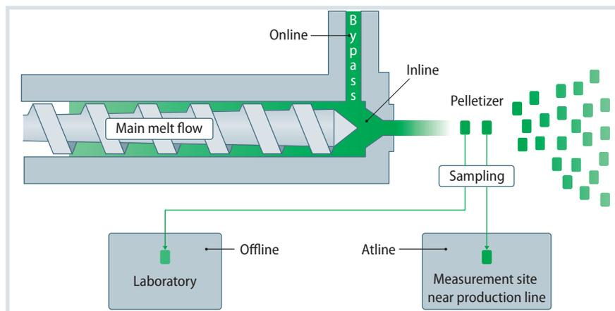
**Fig. 1.** Overview of measurement methods based on a compounding process: inline, online and atline measurements are analysis methods close to the process. Source: SKZ; graphic: © Hanser
