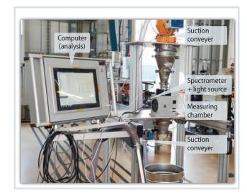
Fig. 2. One of the prototypes is a mobile version that can be used for atline measurement. © SKZ
