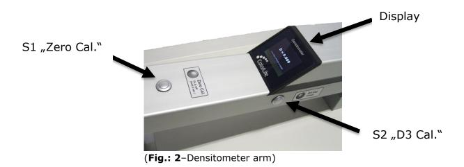
The densitometer is turned on by pressing the S1 button ("Zero Cal."). And is turned off by holding the S1 button down for two seconds, while the arm is an upper position.
