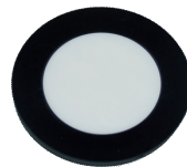
White certified calibration standard
