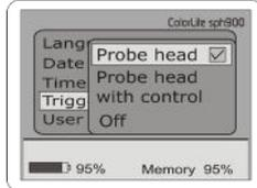
The measurement is triggered by pressing down the outer sleeve of the probe head downwards.
