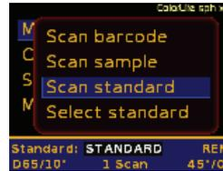
The measurement is triggered by pressing the **“CENTER”** **●** key and following instructions or by pressing the probe head downwards [see chapter 4.9 Probe head handling].
