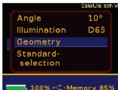
To manually select the probe head adapter, go to "**Settings**" menu and choose "**Geometry**".
