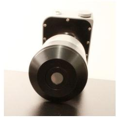
d/8° measurement geometry Measuring area 6 or 10 mm
