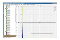
Online window for direct operation of the spectrophotometer from the computer via USB.
