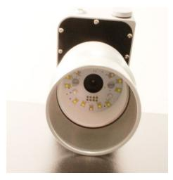
d/0° measurement geometry Measuring area 38 mm
