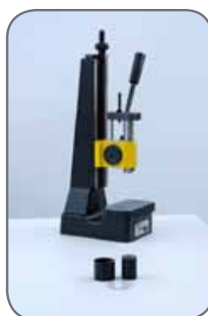
Fig. 2: Powder press with sleeve and plunger
