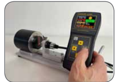
Fig. 1: Transmission measurement with the TA35-UK
