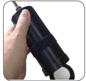
Fig. 1: Probe Head d/0°, Scanning Area: 38 mm for inhomogeneous samples
