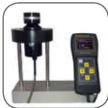
Fig. 3 – black reference on top of the probe head
