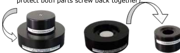
Fig.:1 BAM-standard with black reference cap screwed on
