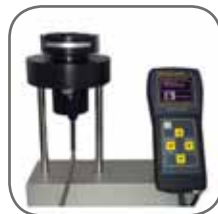
Fig. 4 – BAM-standard on top of the probe head
